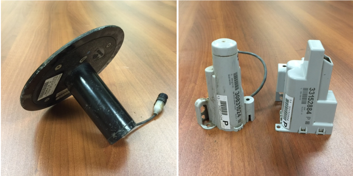
Left is a picture of an Itron 50W-series ERT module and on the Right are Itron 60W-series and 100W-series ERT modules.
