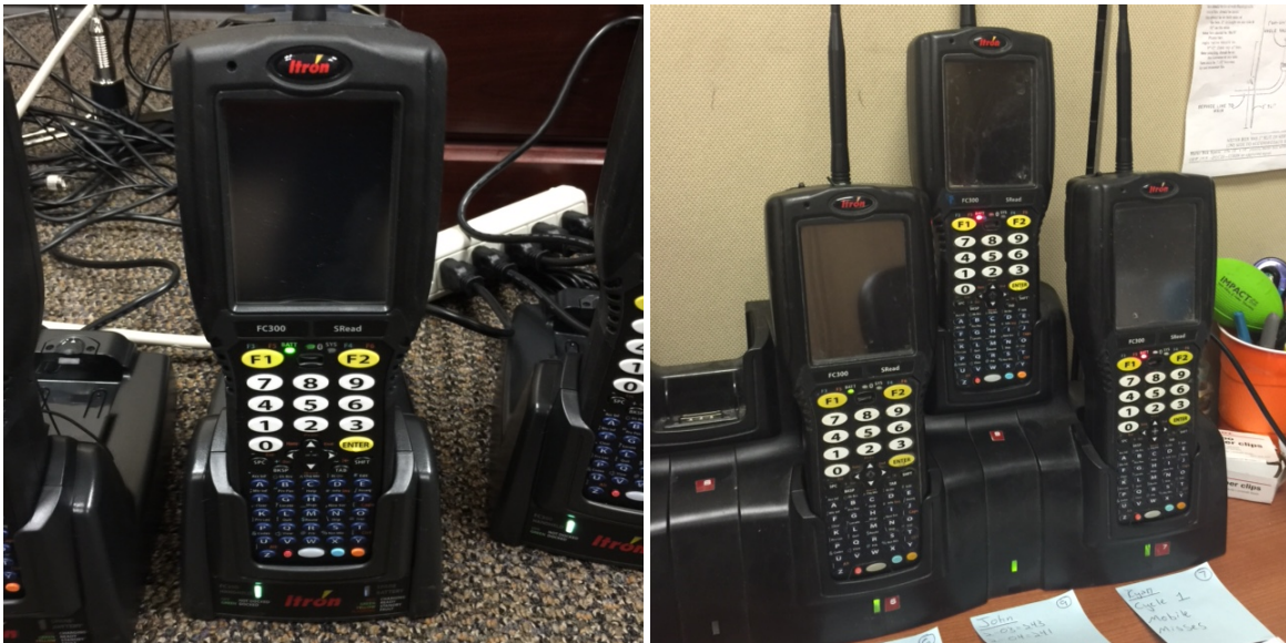
Left is a picture of the FC300 electronic handheld device. On the Right, FC300s in their docking cradle to download daily AMR and manual reads into MV-RS.
