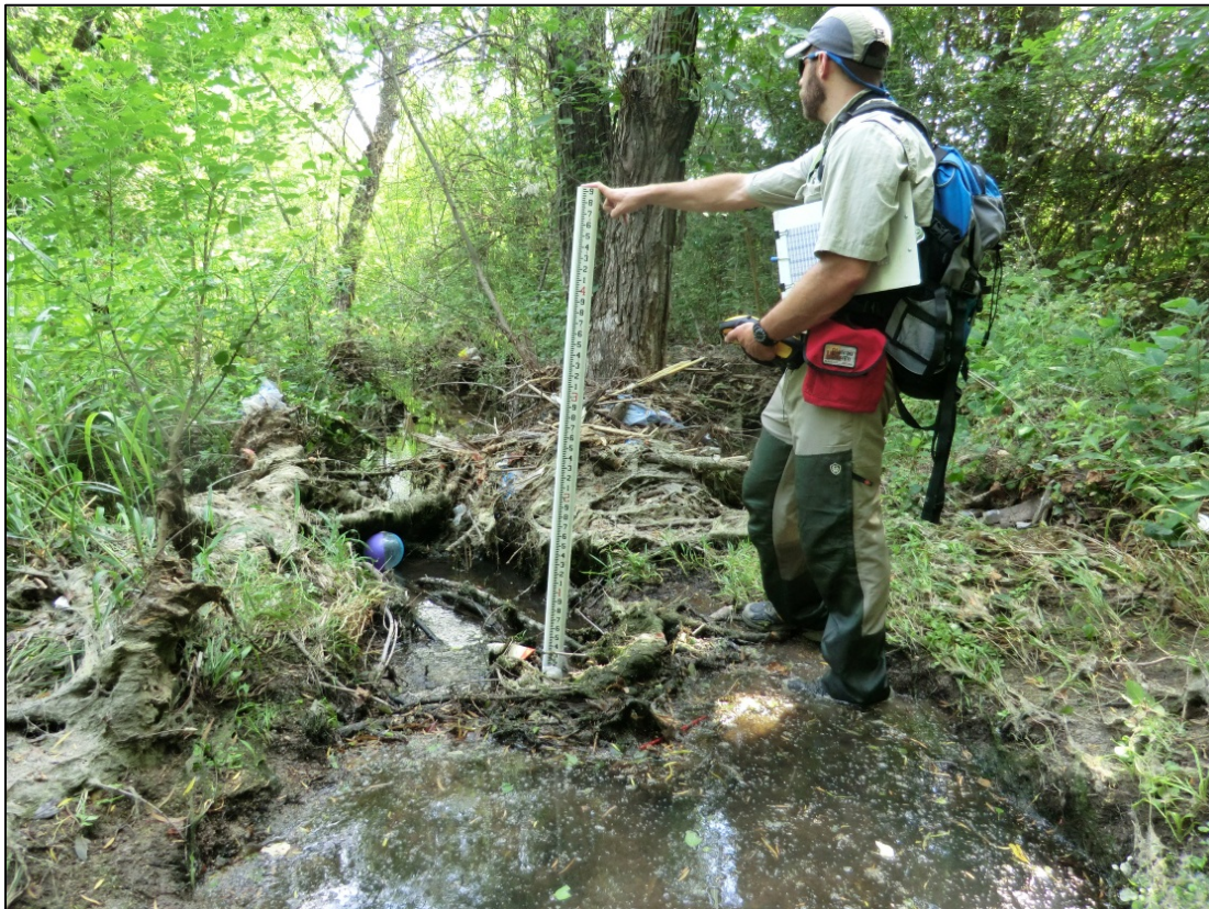
Figure 4.2 Looking downstream near cross section 6056 at a knickpoint with a 1.5-foot drop in elevation.
