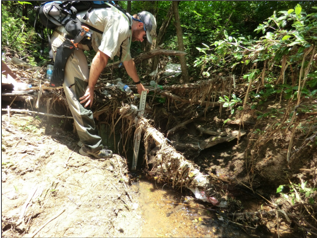
Figure 4.3 Looking downstream near cross section 3491 at a knickpoint with a 2-foot drop in elevation.
