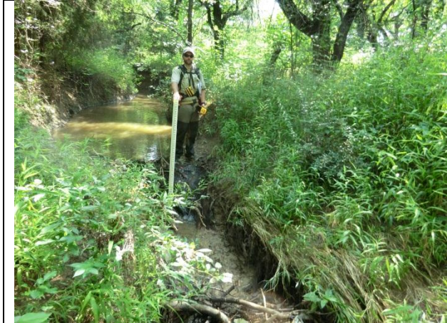
Downstream of 1433 there was a series of knickpoints migrating in the upstream direction.
