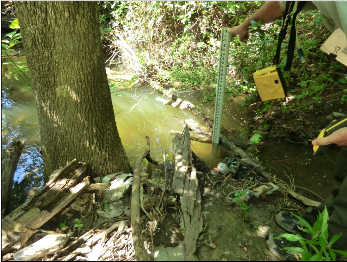
Figure 4.3 Looking downstream near cross section 3778, there was a knickpoint with a 2-foot drop in elevation.
