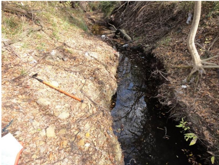
Figure 40. Stream is downcutting into shale. Shale is noted in the bank under the hammer to the left.
