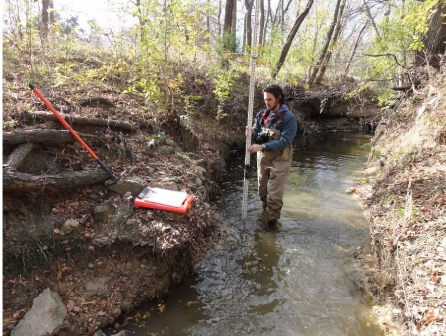
Figure 39. Incising reach. Notebook is on the old channel bottom.
