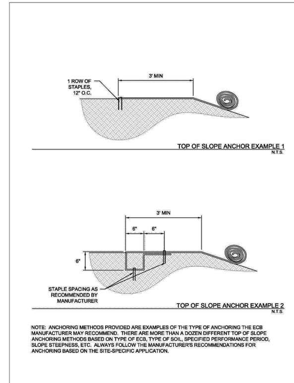
Figure 2.8 Anchor Examples for Erosion Control Blankets
