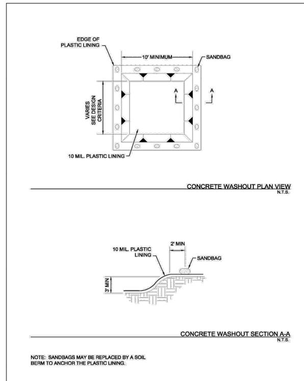
Figure 4.1 Schematics of Concrete Washout Containment
