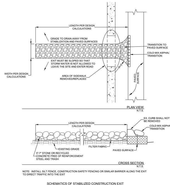
Schematics of Stabilized Construction Exit
