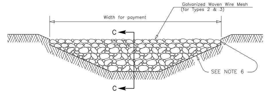
**FILTER DAM AT CHANNEL SECTIONS**
