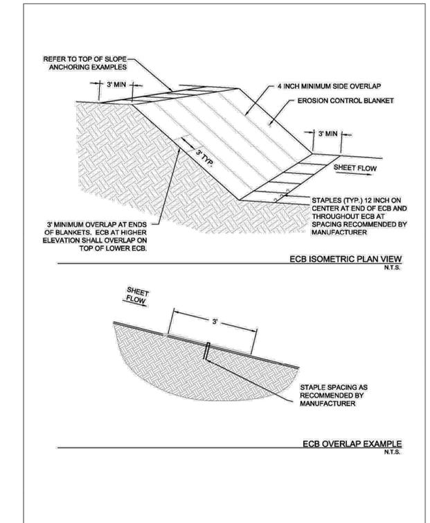
Figure 2.7 Schematics of Erosion Control Blankets
