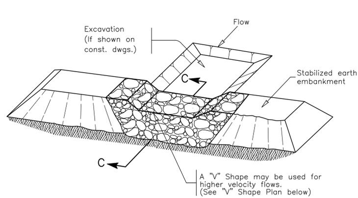
**FILTER DAM AT SEDIMENT TRAP**
