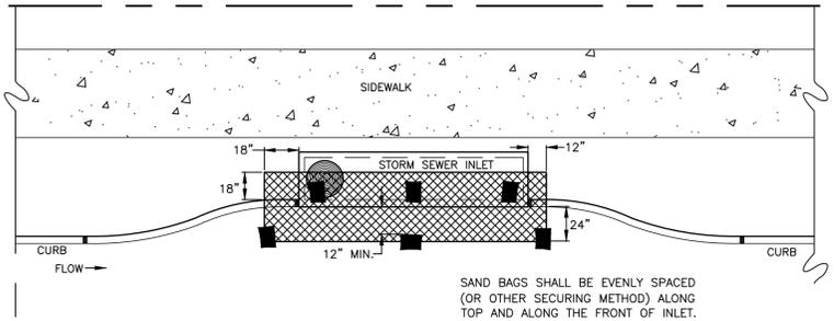
**CURB INLET ON GRADE PROTECTION DETAIL**
